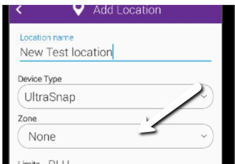
Select and tap the required Zone for the location. Note on the instrument the zones are not listed by number but the full HACCP description.
