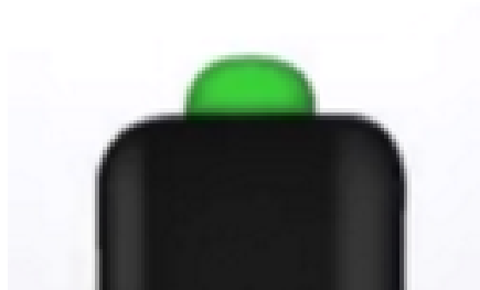
Figure 5. Green light present when rod is activated and receiving sufficient voltage.
