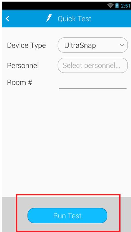
4. If the **Quick Test** screen does not display a **Run Test** button and instead displays a message reading "Insert activated device and close lid," then your instrument needs to be repaired. Contact Hygiena support using the link [here](#).
