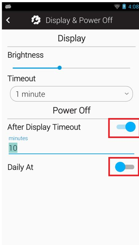
7. To adjust the **After Display Timeout** setting, tap the number under the setting. Enter the number of minutes you want the instrument to wait before powering off. Then tap **Done**.
